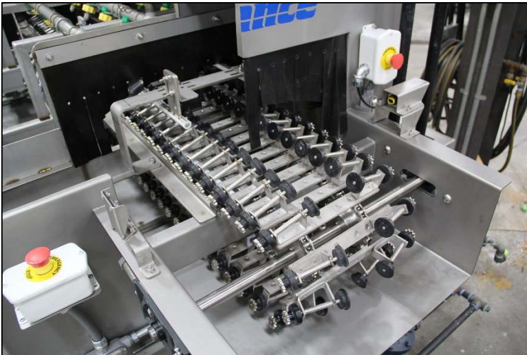
Dual chain with custom rotating fixtures
