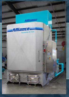
Even large parts can be cleaned in an Alliance cabinet washer. The door is designed to allow parts to be placed in via overhead hoist. A spacesaving roll-in door is also available as an option.
