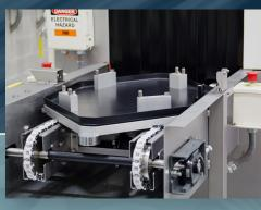
Cleaning system with part fixtures on a chain conveyor
