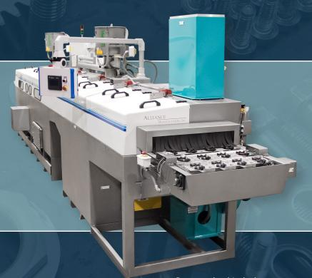
Conveyorized Indexing system with custom part fixtures
