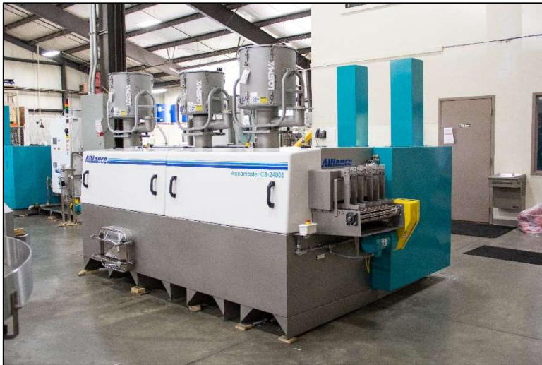
Four-lane cleaning system
