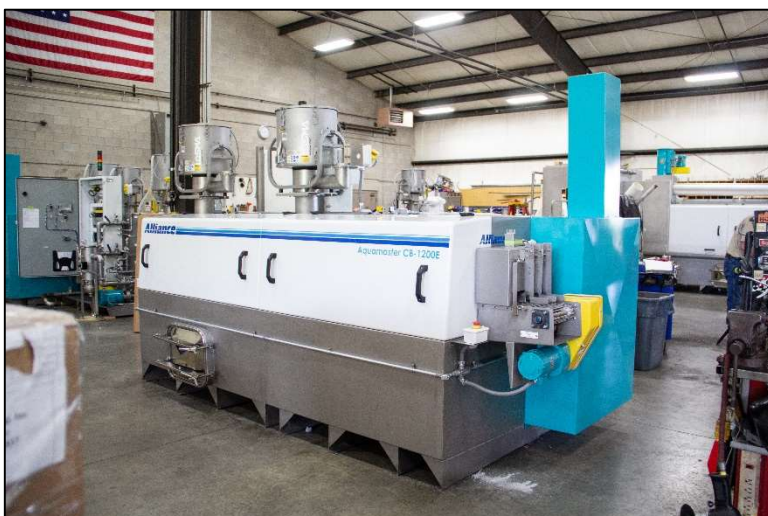
Two-lane cleaning system
